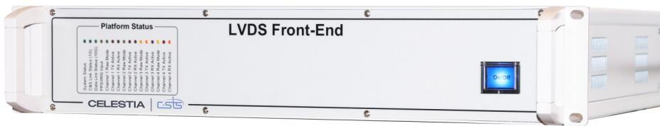
The PLFE provides the electrical, data extraction, protocol handling and status annotation functions. The recovered data (or data to be generated) is offloaded from the PLFE using a 10Gbit TCP/IP streaming interface (SFP+, optical or copper) to a commercial server platform for data storage (or replay) to local disks (SSD or HDD).
