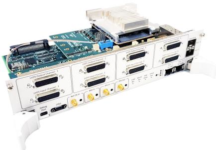
All LVDS in- and outputs are fully isolated (with respect to the chassis/safety ground) and provide satellite level fault voltage emissions and tolerances.
