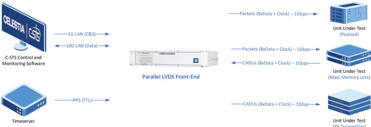
The PLFE parallel LVDS inputs and outputs supports up to four 8-bit data + clock interfaces in parallel, where the clock for each channel can run in excess of 125MHz. In addition it is possible to team two channels to operate as a single 16-bit data + clock interface. Supports flow-control and enable signals.
