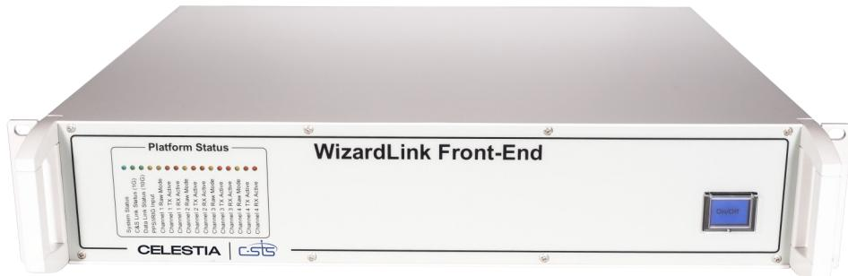
The WLFE provides all electrical, data extraction, protocol handling and status annotation functions. The recovered data (or data to be generated) is offloaded from the WLFE using a 10Gbit TCP/IP streaming interface (SFP+, optical or copper) to a commercial server platform for data storage (or replay) to local disk.
