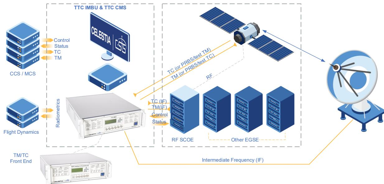
The internal processing allows the modulation to be fed by external signals (e.g. via RS422) or internal sources such as an ITU compatible PRBS generator, Telecommand generator or Telemetry Simulator with or without ranging uplink signals. Likewise the Demodulation output can be output to external equipment (e.g. via RS422) or further processed within the TTC IMBU including Telemetry data acquisition, frame synchronization, Viterbi/ Reed-Solomon error correction etc.)
