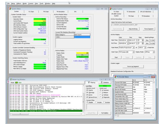
TM/TC Interface & Processing Unit (IPU) combined with the Control and Monitor Software (CMS) running on a workstation/PC.
