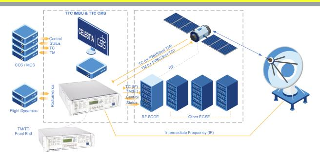
The internal processing allows the modulation to be fed by external signals (e.g. via RS422) or internal sources such as an ITU compatible PRBS generator, Telecommand generator or Telemetry Simulator with or without ranging uplink signals. Likewise the Demodulation output can be output to external equipment (e.g. via RS422) or further processed within the TTC IMBU including Telemetry data acquisition, frame synchronization, Viterbi/Reed-Solomon error correction etc.)
