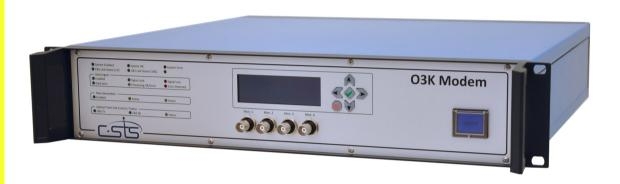
The O3K Modem processing is based on the (currently evolving) CCSDS O3K recommendations. However, all processing can be adapted as needed by C-STS for a specific application.
