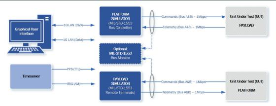
The MIL-1553 Front-End can be configured to act as: Bus Controller, Bus Monitor or Remote Terminal Simulator.
