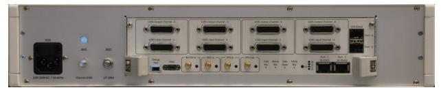
All LVDS in— and outputs are fully isolated (with respect to the chassis/safety ground) and provide satellite level fault voltage emissions and tolerances. The unit is provided with an FMEA report.
