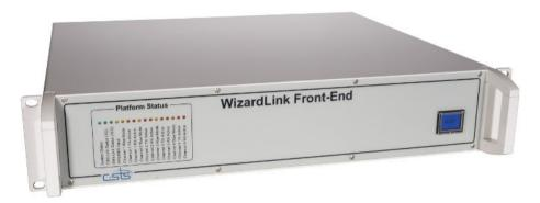
The WLFE provides all electrical, data extraction, protocol handling and status annotation functions. The recovered data (or data to be generated) is offloaded from the WLFE using a 10Gbit TCP/IP streaming interface (SFP+, optical or copper) to a commercial server platform for data storage (or replay) to local disk.
