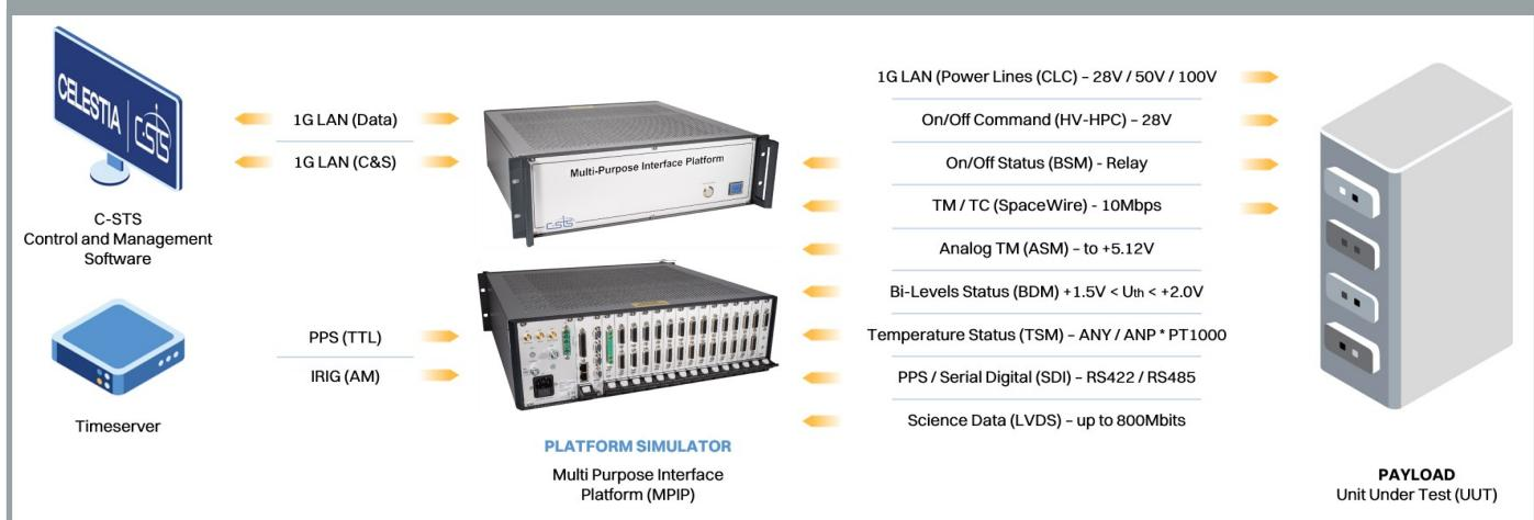
The MPIP is a versatile system that can be used to test and/or simulate electrical interfaces of spacecraft sub-systems such as:
