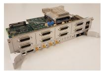
The Parallel LVDS Front-End is part of the suite of latest generation EGSE products from C-STS that provides a wide range of onboard interface front-ends, such as Discretes, Power (LCL), RS-422 (SDI), CAN, MIL-STD-1553, SpaceWire, WizardLink, SpaceFibre and many more.
